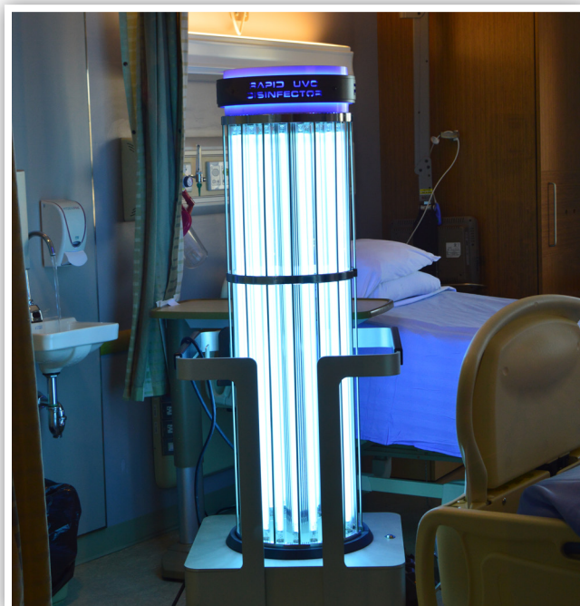
Picture of ultraviolet light disinfection system in a patient room. Please note, this picture was taken for demonstrational purposes only and during and actual room cleaning the bedding is removed during the UV cleaning process.
